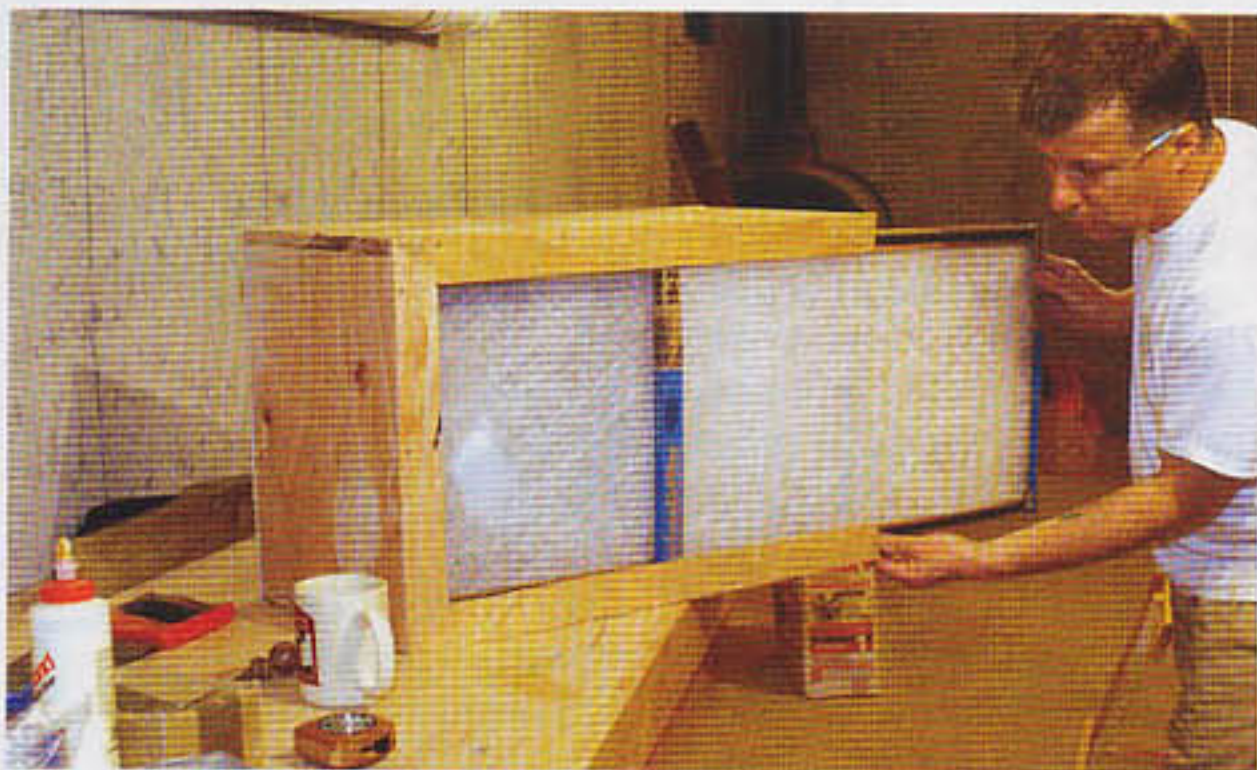
The ply cabinet is designed to accept the disposable filters which simply slide into place. They will trap particles down to 1 micron
